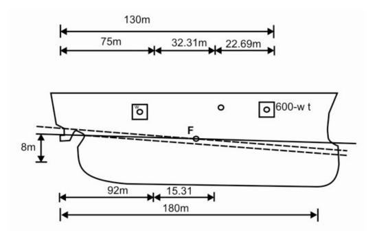
TCP, 23 tonne/cm; MCTC, 180 tonne/cm; LCF, 92m forward of AP; length 180m. Distance of centre of gravity of weight from LCF
