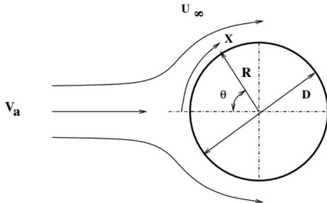
The objective is to determine point of separation  $x_{sep}^*$  corresponding to  $\kappa = -0.1567$ .
