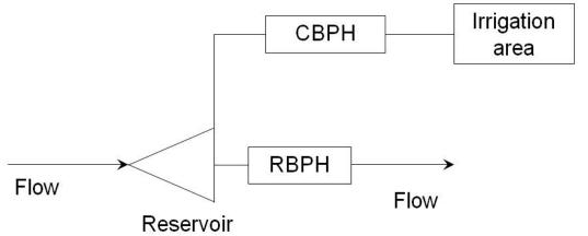
CBPH: Canal Bed Powerhouse RBPH: Riverbed Powerhouse
