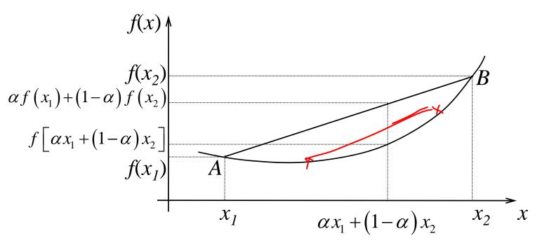
A straight line (AB) drawn between any two points is above the curve
