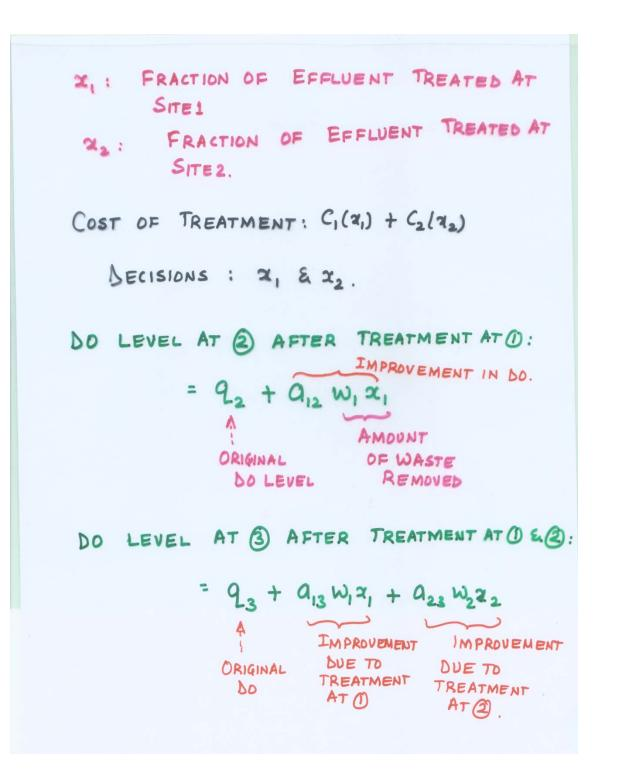
OPTIMIZATION MODEL: MIN.  $C_1(x_1) + C_2(x_2)$ - Jesned @ 2 S.t.  $x_{min} \leq x_1 \leq x_{max}$ Xmin S X2 S Xmax. TECHNOLOGICAL LIMITS 5
