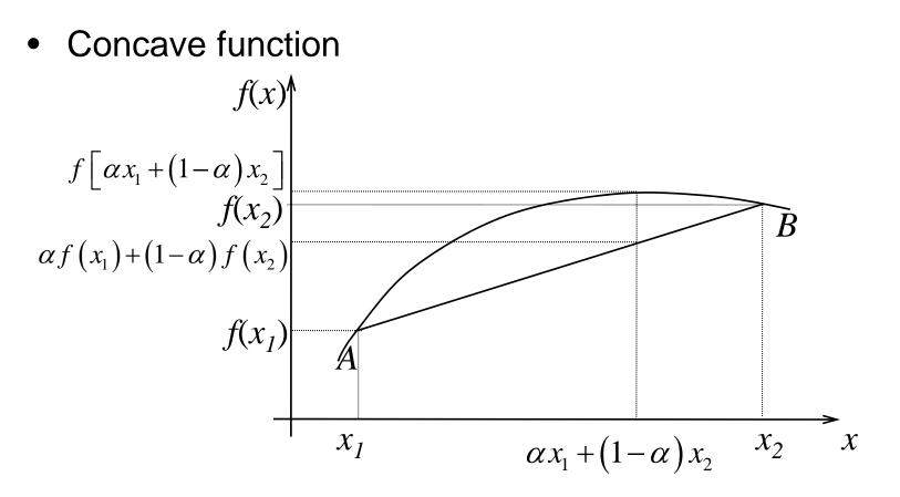
A straight line (AB) drawn between any two points is below the curve
