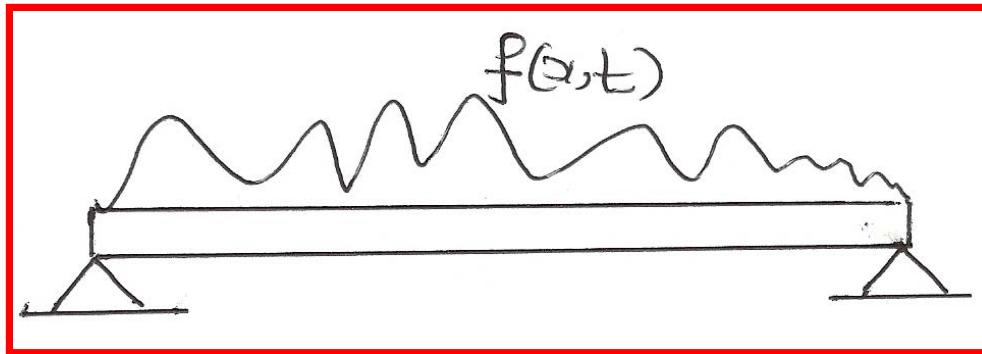
$$\frac{\partial^2}{\partial x^2} \left[ EI(x) \frac{\partial^2 y}{\partial x^2} + \nu EI(x) \frac{\partial^3 y}{\partial x^2 \partial t} \right] + m(x) \ddot{y} + c(x) \dot{y} = \underline{\underline{f(x,t)}}$$
