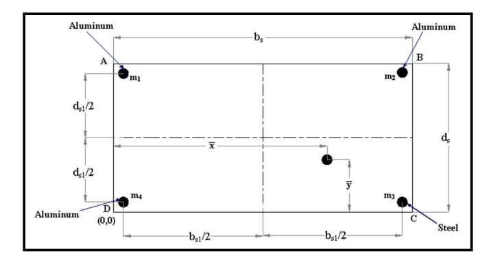
$$\overline{x} = \frac{m_s \frac{b_s}{2} + (m_1 + m_4) \left(\frac{b_s - b_{s1}}{2}\right) + (m_2 + m_3) \left(\frac{b_s + b_{s1}}{2}\right)}{\rho_s t b_s d_s + m_1 + m_2 + m_3 + m_4}$$
