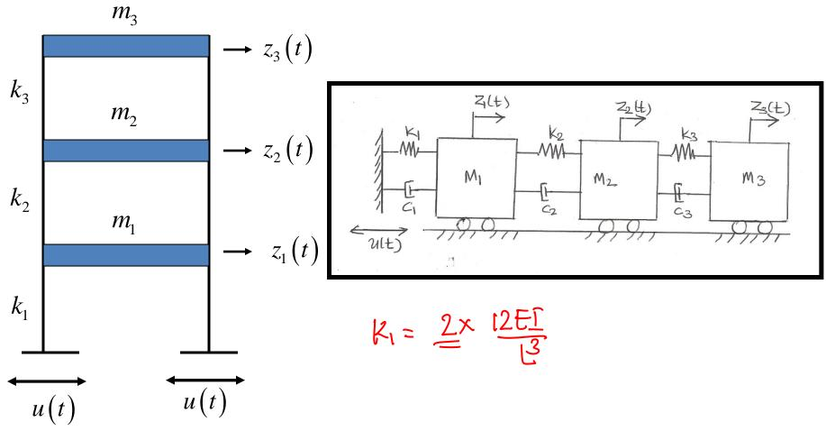
$$\begin{array}{c|c} k_{1}(z_{1}-z_{1}) \leftarrow & k_{2}(z_{1}-z_{2}) \\ M_{1} \notz_{1} \leftarrow & M_{1} \\ c_{1}(z_{1}-\dot{u}) \leftarrow & M_{1} \\ c_{2}(z_{1}-\dot{u}) \leftarrow & c_{2}(z_{1}-\dot{z}_{2}) \\ \end{array}$$
