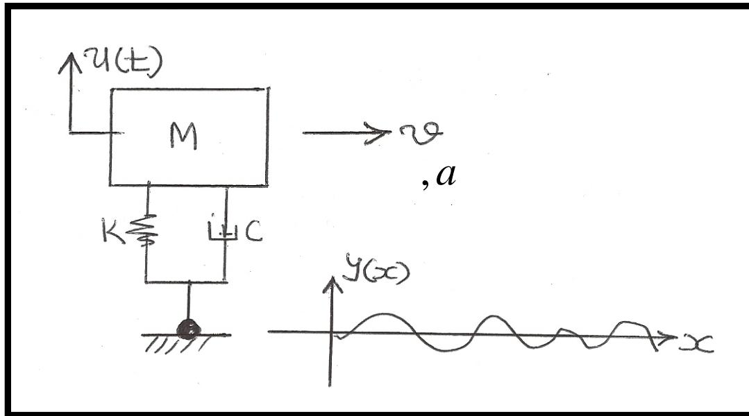
$$m\ddot{u} + c \frac{d}{dt} \left[ u - y(x = vt + 0.5at^2) \right] + k \left[ u - y(x = vt + 0.5at^2) \right] = 0$$
