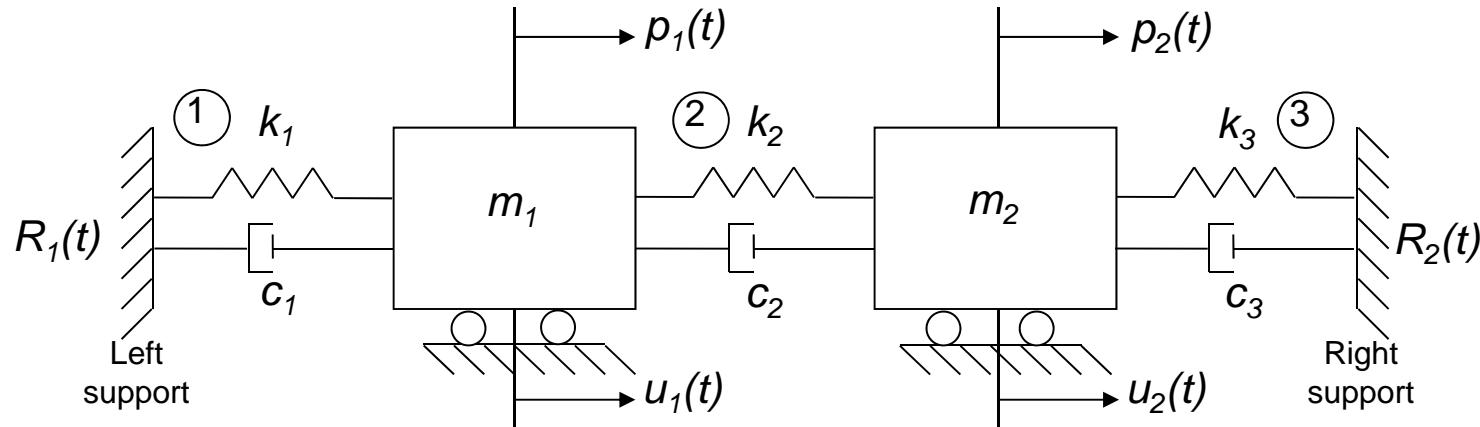
Springs  $k_1$  and  $k_2$  have cubic force displacement characteristics and spring  $k_3$  is an inelastic spring modeled using Bouc's approach.
