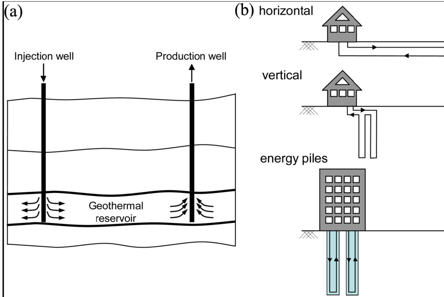
fig: Geothermal Systems: (a) Deep Geothermal Recovery for Electricity Generation, (b) Distributed Geothermal Storage/ Recovery Systems at Shallow Depth for Residential Purposes
