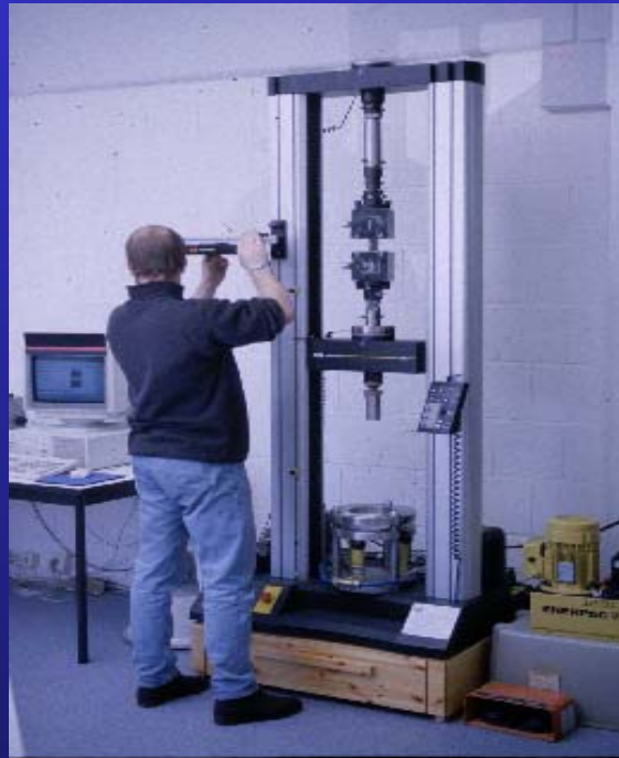
Testing machine with video-extensometer
