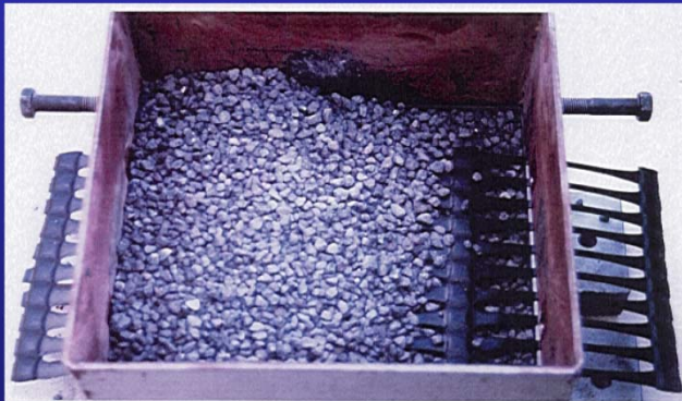
Filling Corundum into upper box
