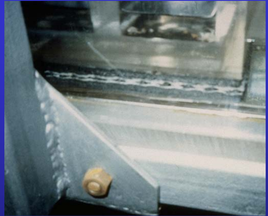
Specimen in apparatus, net core with soft contact faces
