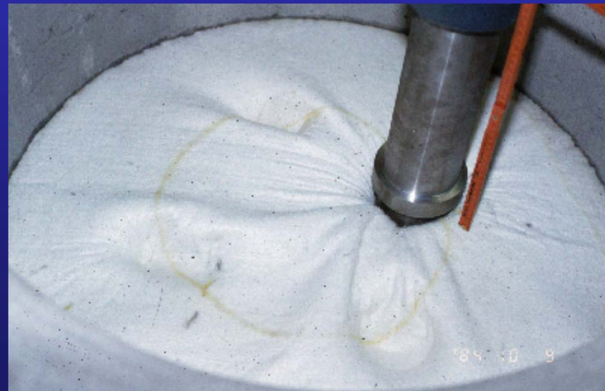
Result of drop tests - no penetration
