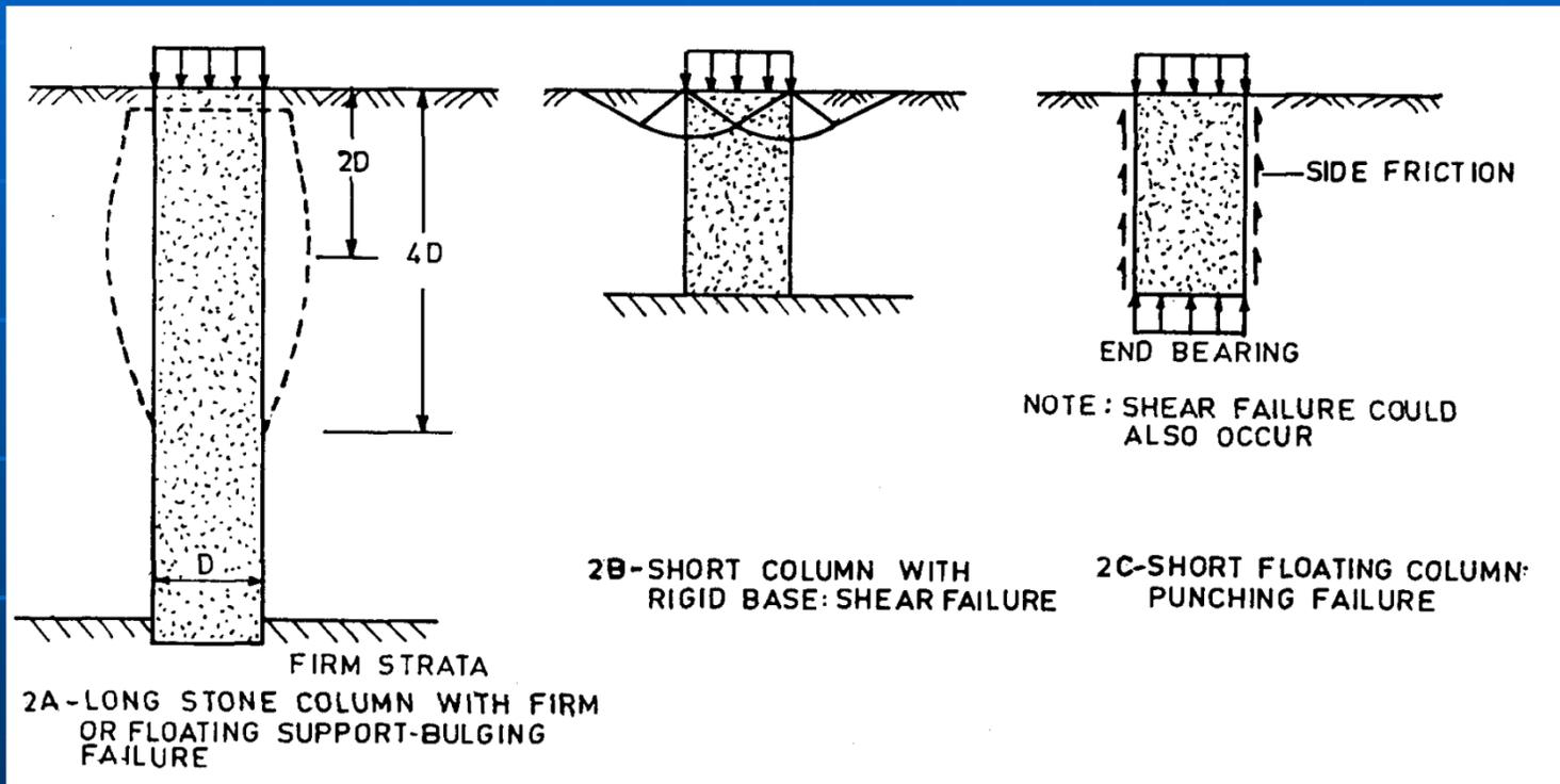
Fig1(a): Failure Mechanism of Single Stone Column in a Homogenous Soft Layer.
