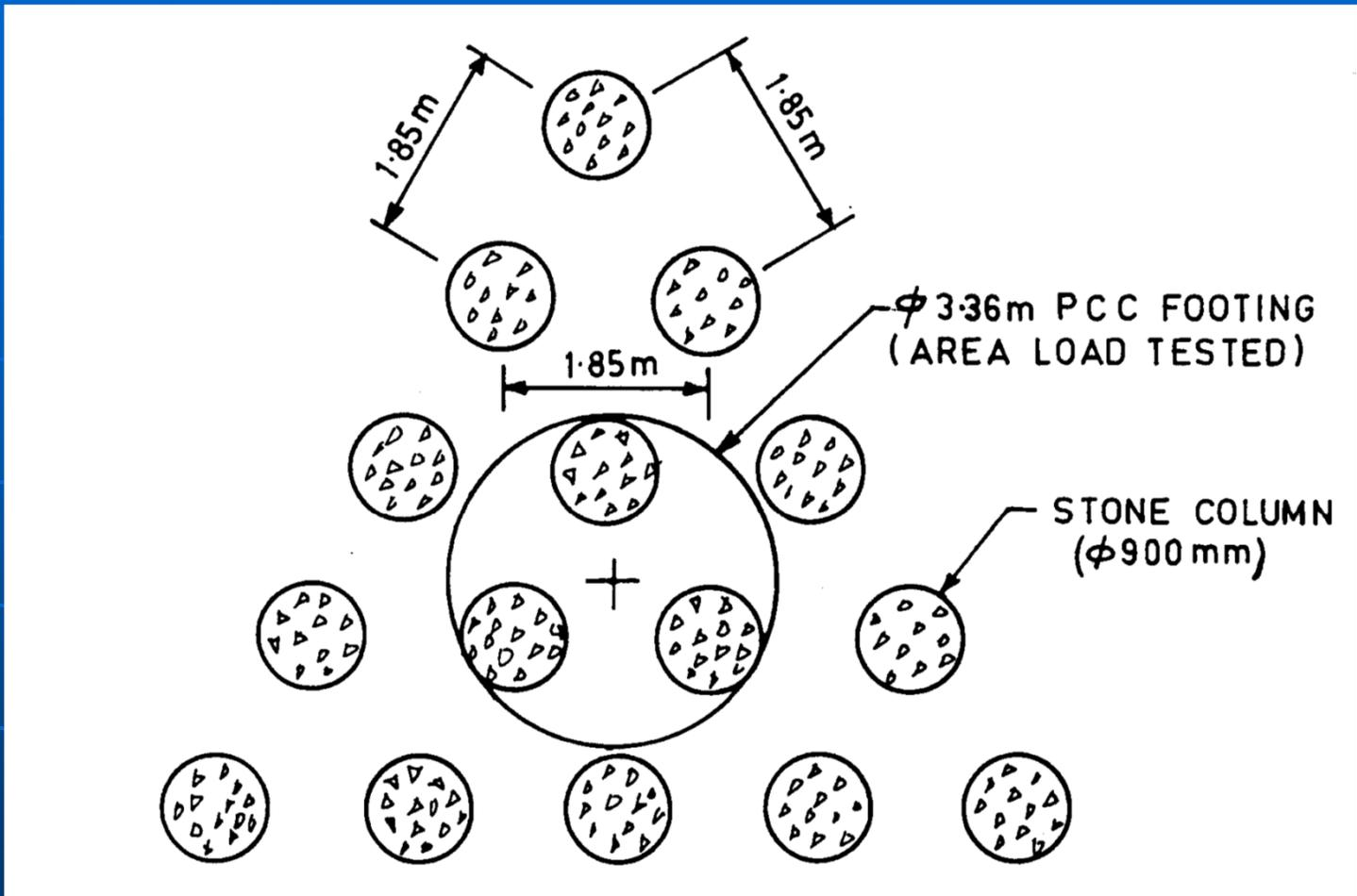
Fig1(d): Load test on Three columns( Group Test).
