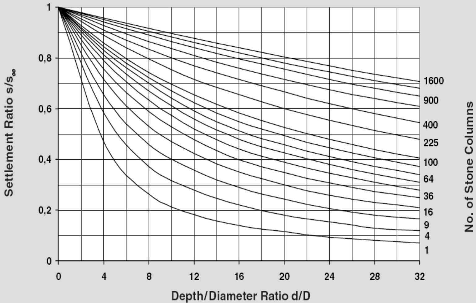
Fig1(e): Variation of settlement ratio with  $d/D$  ratio of Single Footing
