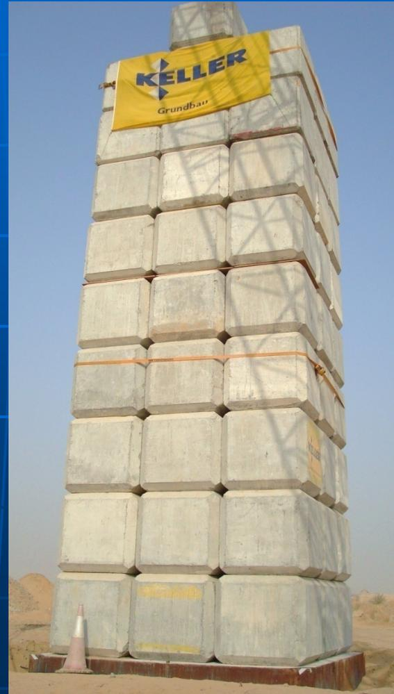
**400 Tons load on 4m x 4m ~ 250 kPa**
