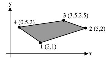
7. For the element shown in the following figure, the solution at the nodes is given as follows:
