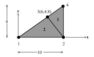
5. Find the lowest eigenvalue  $\lambda$  for the following problem using two linear triangular elements as shown in the following figure.
