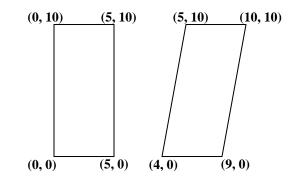
11. Compute stresses and strains at a point located at (2,2) for the problem shown in the following figure, using only one quadrilateral element. Assume plane strain conditions. E = 20.6842GPa, v = 0.25, thickness = 0.0254 m.
