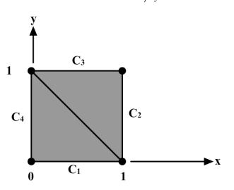
4. Obtain an approximate solution of the following boundary value problem using two linear triangular elements as shown in the following figure.
