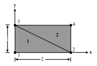
2. Obtain an approximate solution of the following boundary value problem using two linear triangular elements as shown in the following figure.
