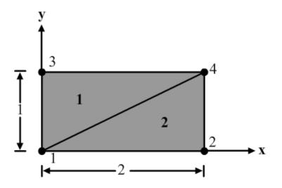
6. Obtain explicit expressions for isoparametric mapping for the element shown in the following figure. Is the mapping is fine? Compute the derivatives  $\partial N_4 / \partial x$ , and  $\partial N_4 / \partial y$ .
