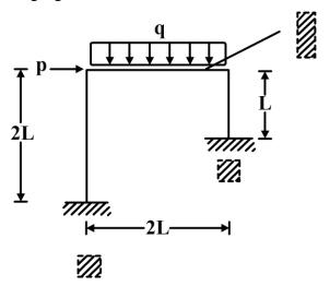
Determine nodal displacements and element forces in a three dimensional frame shown in the following figure. The beams are of rectangular cross section 0.254 m × 0.381 m. The column is of square cross section 0.254 m × 0.254 m. Assume L = 4.572 m, q = 29.1878 N/m, P = 44.482 kN, E = 20.6842GPa, G = 6.895 GPa.
