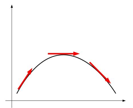
Positive slope Zero slope Negative slope
