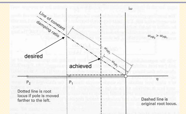
Moving pole  $P_1$  to  $P_2$  is impractical, unless there is an increase in wingspan of the aircraft..! Hence, the cure is to have a stability augmentation system.
