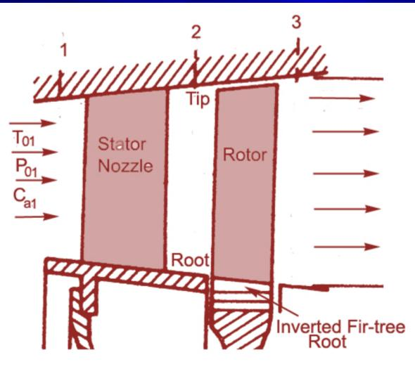
Elemental Turbine stage – Rotor + Stator
