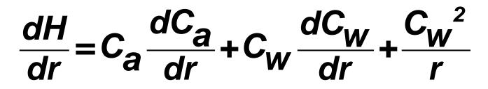
• At entry to the compressor, except near the hub and the casing, enthalpy H (r) = constant.
