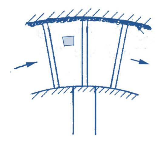
Let us assume that a small element inside the rotating blade passage represents the fluid flow inside the rotor, such that the analysis of the status of this element may wholly represent the status of the whole flow inside the rotor passage
