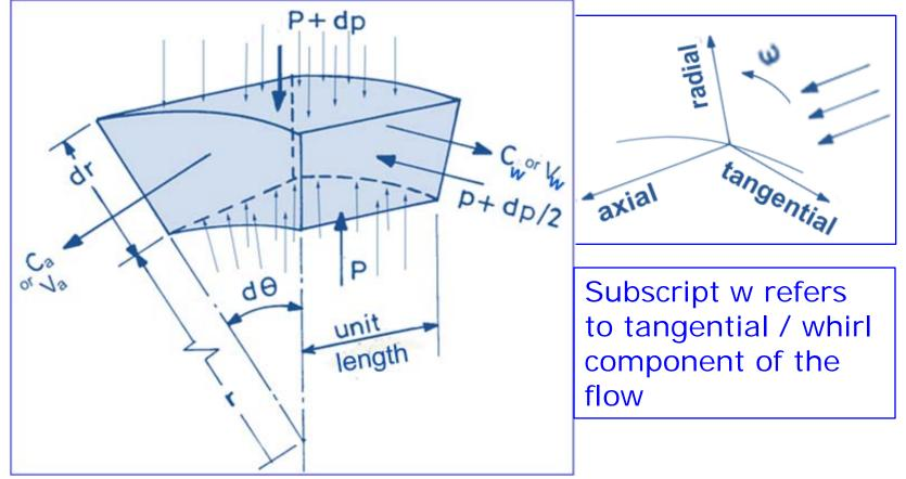
Resolving all the aerodynamic forces, acting on this element, in the radial direction,
