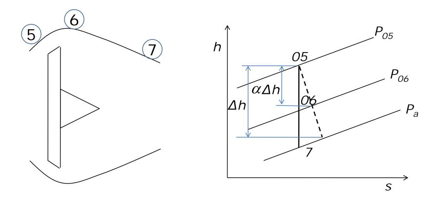
Enthalpy-entropy diagram for power turbineexhaust nozzle analysis
