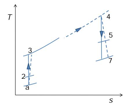
Real turbojet cycle (without afterburning) on a T-s diagram
