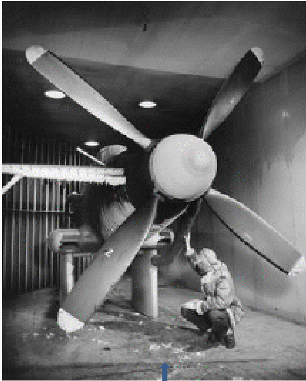
Propeller undergoing a wind tunnel testing
