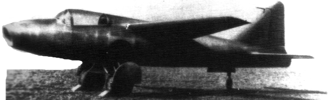
Heinkel He 178 First Jet engine powered aircraft
